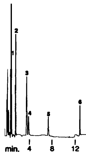
Figure 11 - Achieve baseline resolution of EPA Method 501.3 and 504 analytes on a 30m, 0.53mm ID, 2.0um Rtx"-Volatiles in less than 13 minutes.
