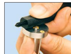
Use the flat side of the Piston Seal Insertion Tool to seat a Waters face seal.
