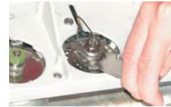
Use the larger end to tighten the split/splitless weldment nut.
